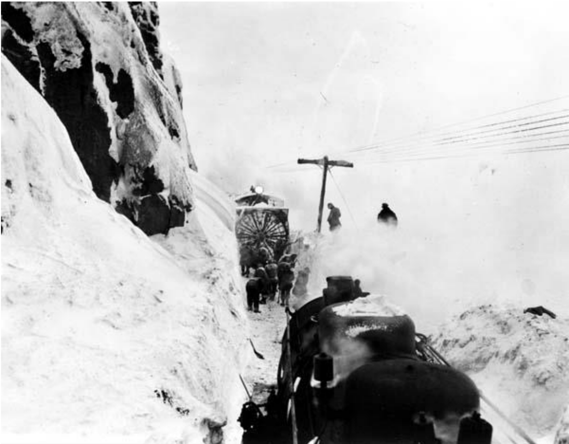
Get it back on the rails boys. W.P. &Y.R. Snowplow clearing tracks after terrific snowstorm. Yukon Archives. William J. Preston fonds, #23.
