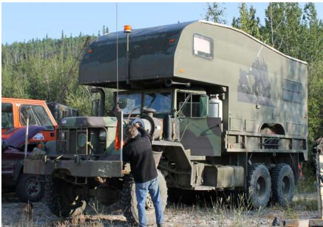
This oversized camper was created by loading a small fifth wheel onto a 5-ton truck. Photo courtesy Dan Davidson uffish@northwestel.net (In Dawson)
