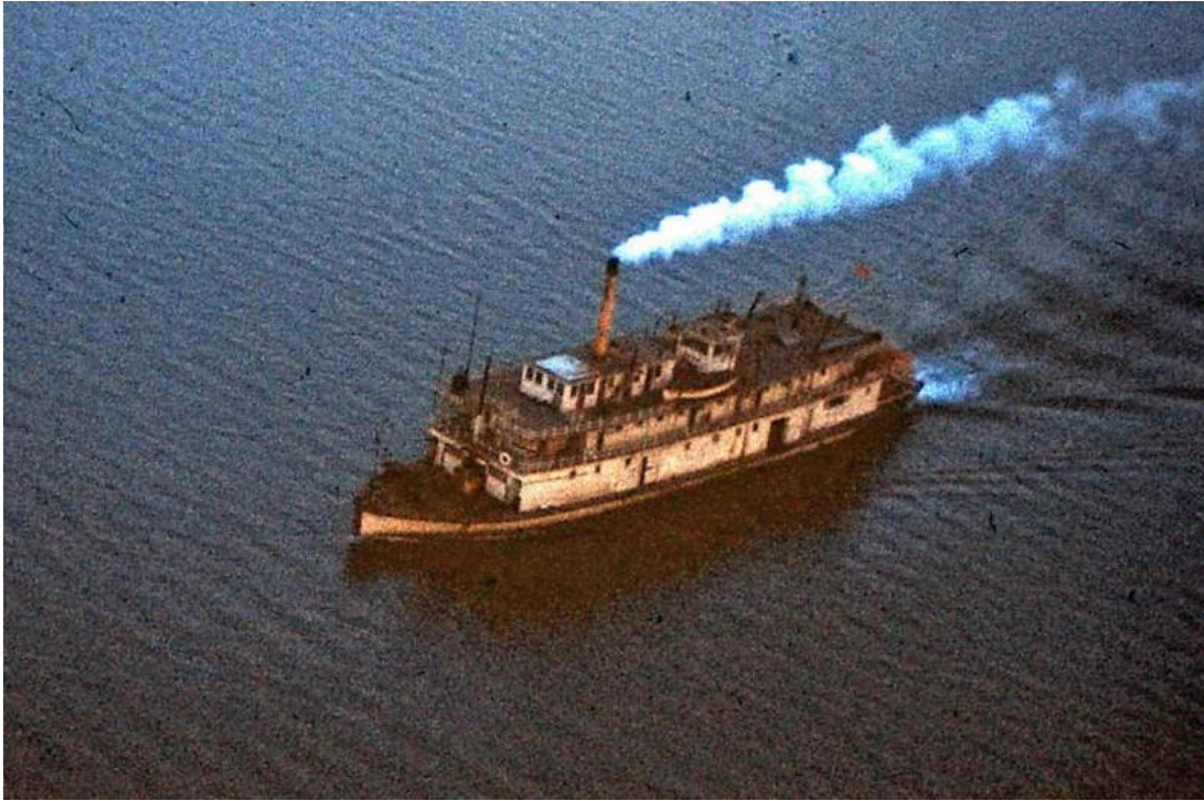
View from the air of her crossing Lac Labarge - Note the wheelhouse removed and placed behind the upper deck in order for her to get under the new Carmacks bridge. The smoke stack was hinged down for that passage also. – August 1960 Photos courtesy Ira Saunders sandisaunders@rogers.com (In Ottawa)
