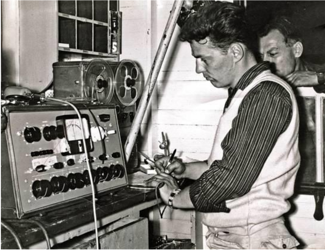
Terry Delaney working in the temporary studio set up on board - compiling a radio report on the progress of the voyage. Equipment Terry is using there is a McCurdy SS1000 audio console and an Ampex 601 Tape Recorder. CBC Yukon technician Ed Kerry is looking on over Terry's shoulder. The Keno spent 3 nights on the river.
