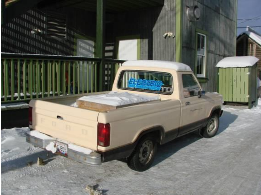
Peter Menzies' Ford Ranger, known as EV2. The box in the truck bed holds the batteries which make it run.
