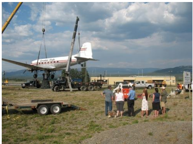
This was scary – the small crane jerked the tail up and down to break the weld cut
