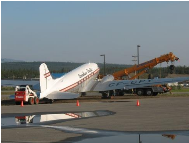
Using bobcat for final positioning before the lift
