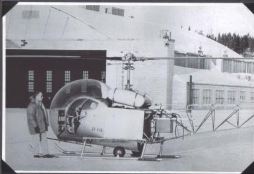
Chuck Hankins with Trans North's first helicopter – the wooden rotor bladed Bell 47G-2, CF-ETR, shown here with winter cowls installed.
