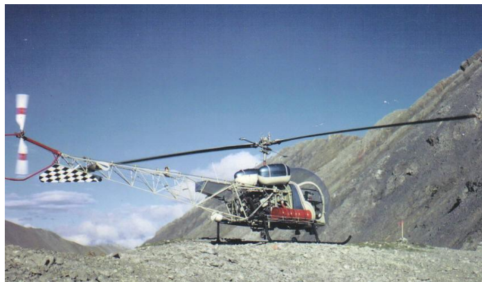
Bell 47 helicopter, the type I flew the first few years on helicopters
