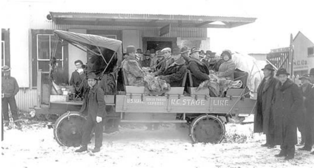
Jeffery_Fairbanks - The Fairbanks News-Miner reported in 1914 that 4 new Jeffery Quads were ordered by the Fairbanks Northern Commercial Company for use in freighting out on the trail. This was one of them (not the one in Eagle, as far as we know).
