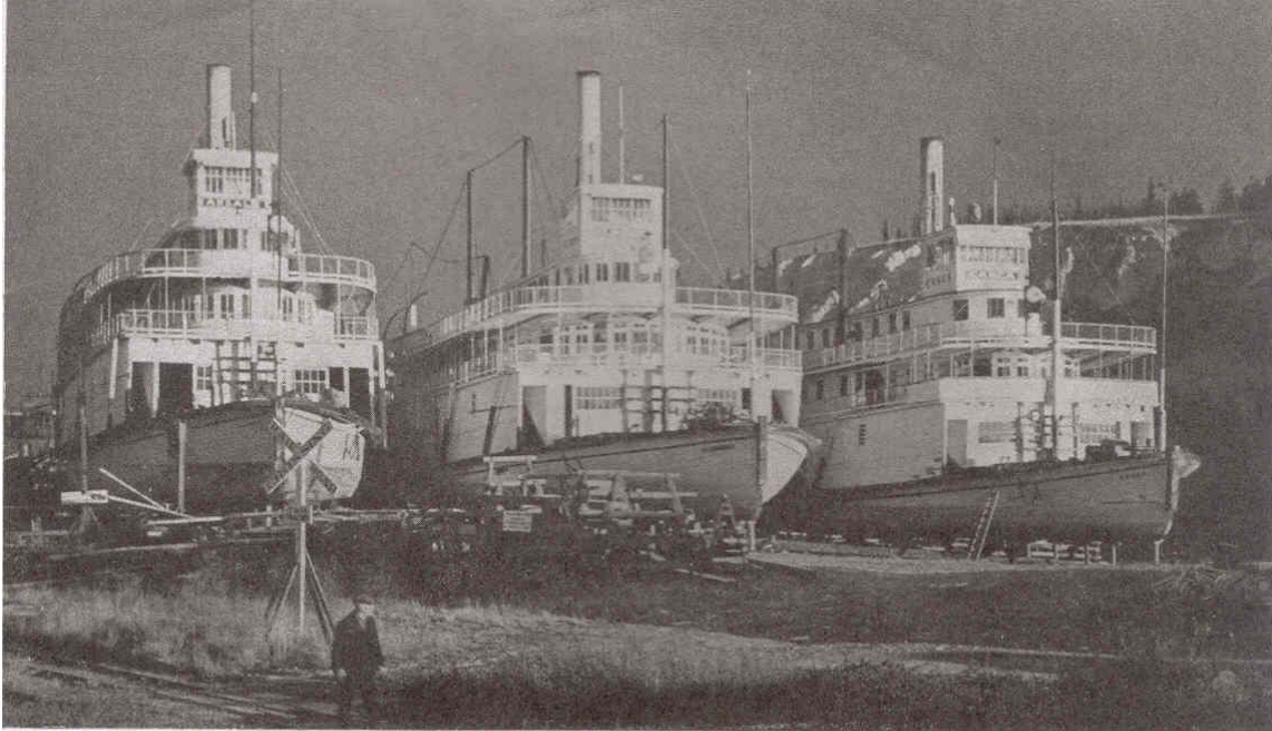
These passenger and cargo stern-wheelers are reminders of the pioneer Yukon days. In summer the boats ply along the Lewes River as they did half a century ago. Hauled ashore for the winter they are repaired to be ready for the navigation season
