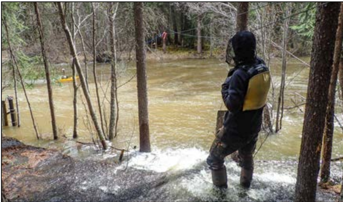
Devon O'Connor manoeuvring a boat-mounted Acoustic Doppler Current Profiler during spring freshet flow measurement on Tay Creek. Photo: Alexandre Mischler.
