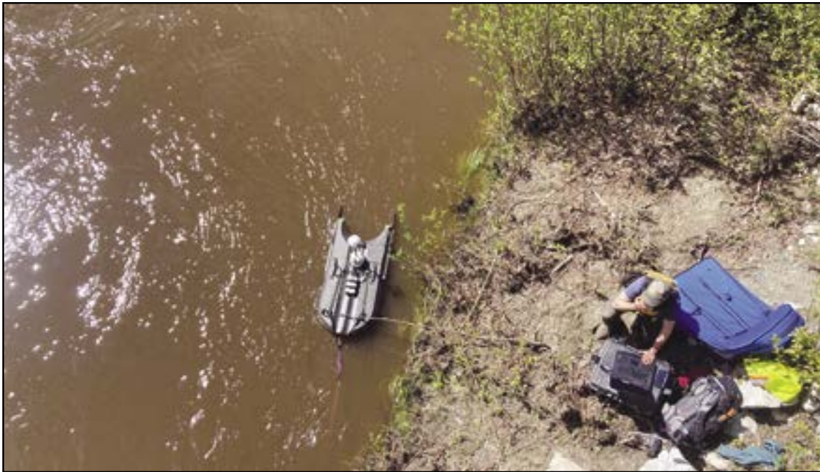
Jonathan Kolot configuring a boat-mounted Acoustic Doppler Current Profiler on Koidern River. Photo: Alexandre Mischler.
