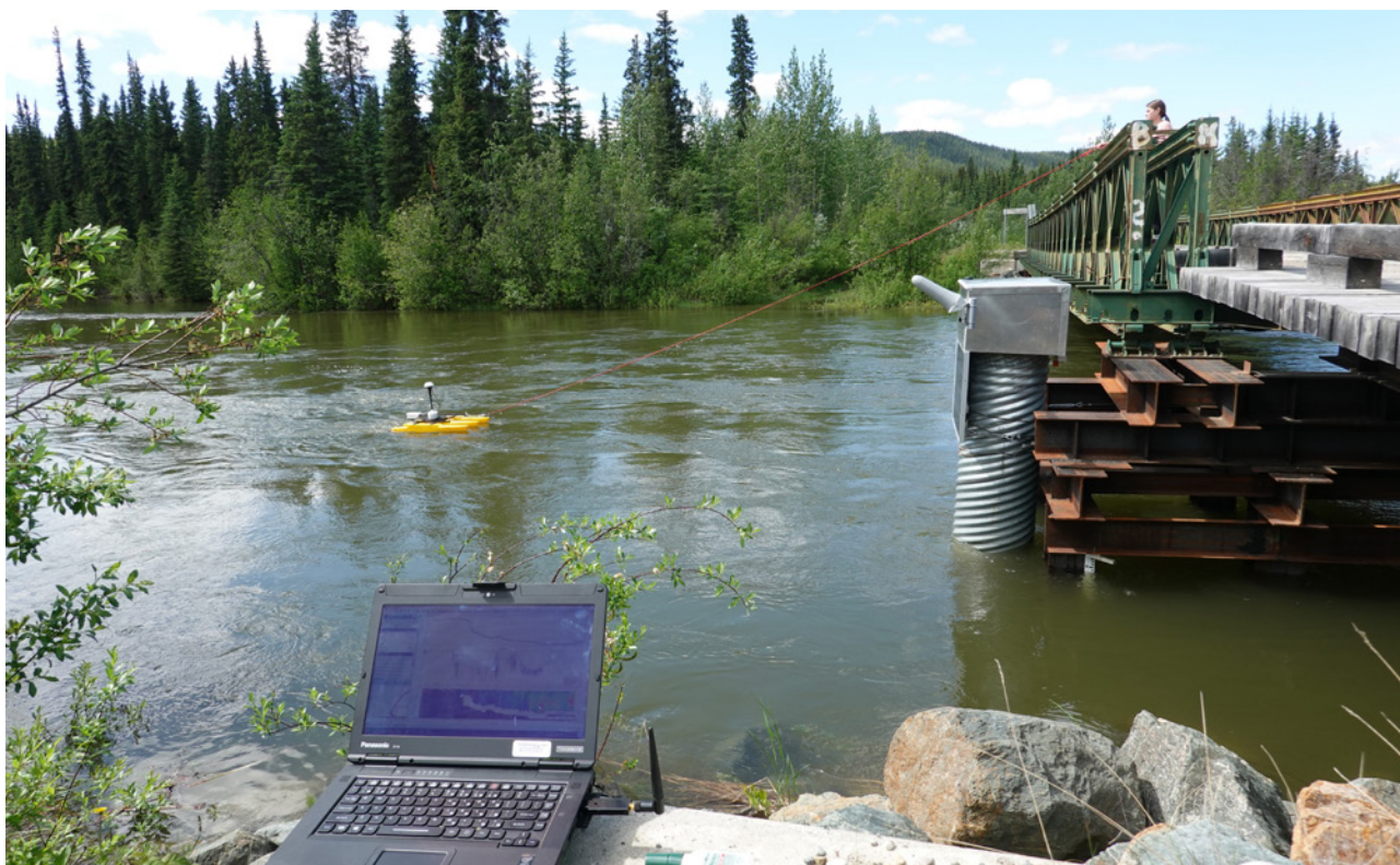
High flow measurement at Ross River Bridge #1 hydrometric station with Acoustic Doppler Current Profiler (ADCP) instrument.
