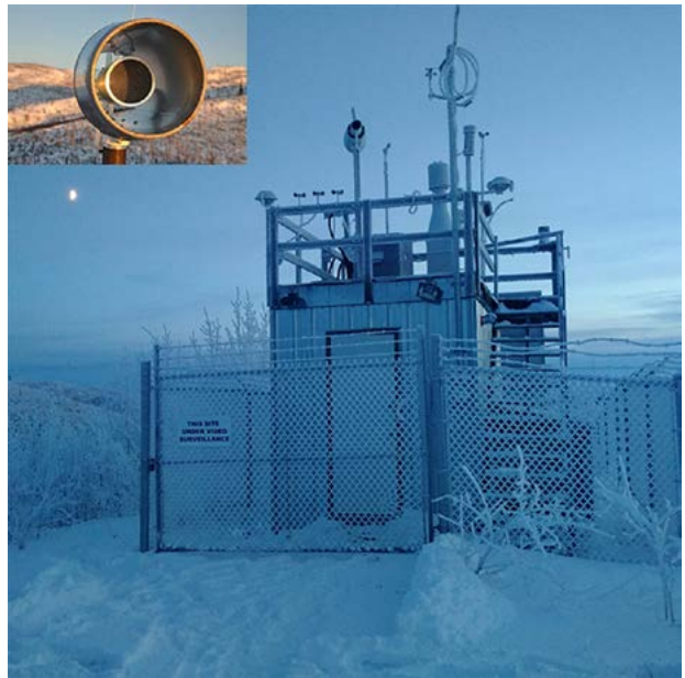
Air monitoring station at Little Fox Lake (inset: flow-through air sampler).
