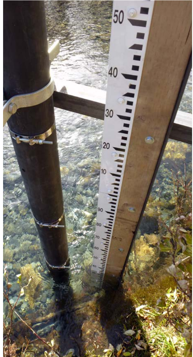
Measuring water levels on 180 Mile Creek.
