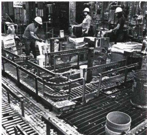
Asbestos bagging operation at Clinton Creek
