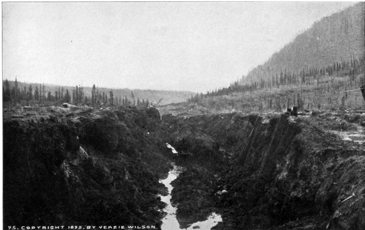
GROUND SLUICING. This is done without any sluice boxes, the water being turned right on the ground, washing away the dirt and leaving the gold.
