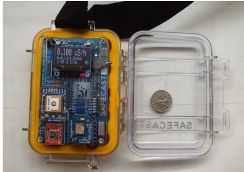
Gerry's bGeigie Nano mobile radiation monitor, which can be mounted to a car to collect radiation measurements. photo: Gerry Whitley
