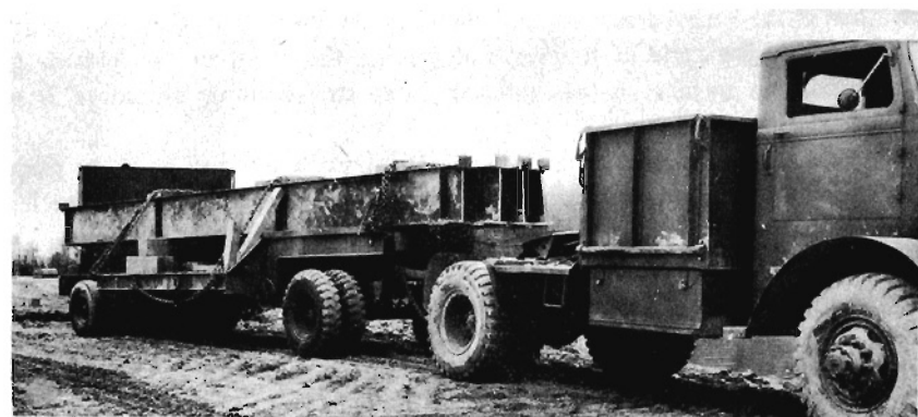
Figure 38. Steel-stringer sections loaded on a trailer. Timbers level the beams and chains and shoring secure the load. Stringers shown are for a 30-foot-span semipermanent highway steel bridge.
