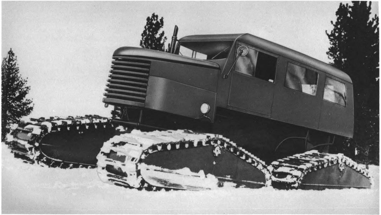
FIGURE 4A1-8 Commercial Cargo and Personnel Carrier (Snow-Cat), 4-Track-Drive, 1½-Ton Payload Capacity
