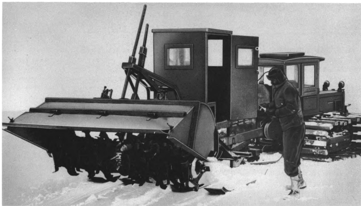
FIGURE 4C2-4 Pulvimixer, Runner-Mounted, Towed by Class I Tractor
