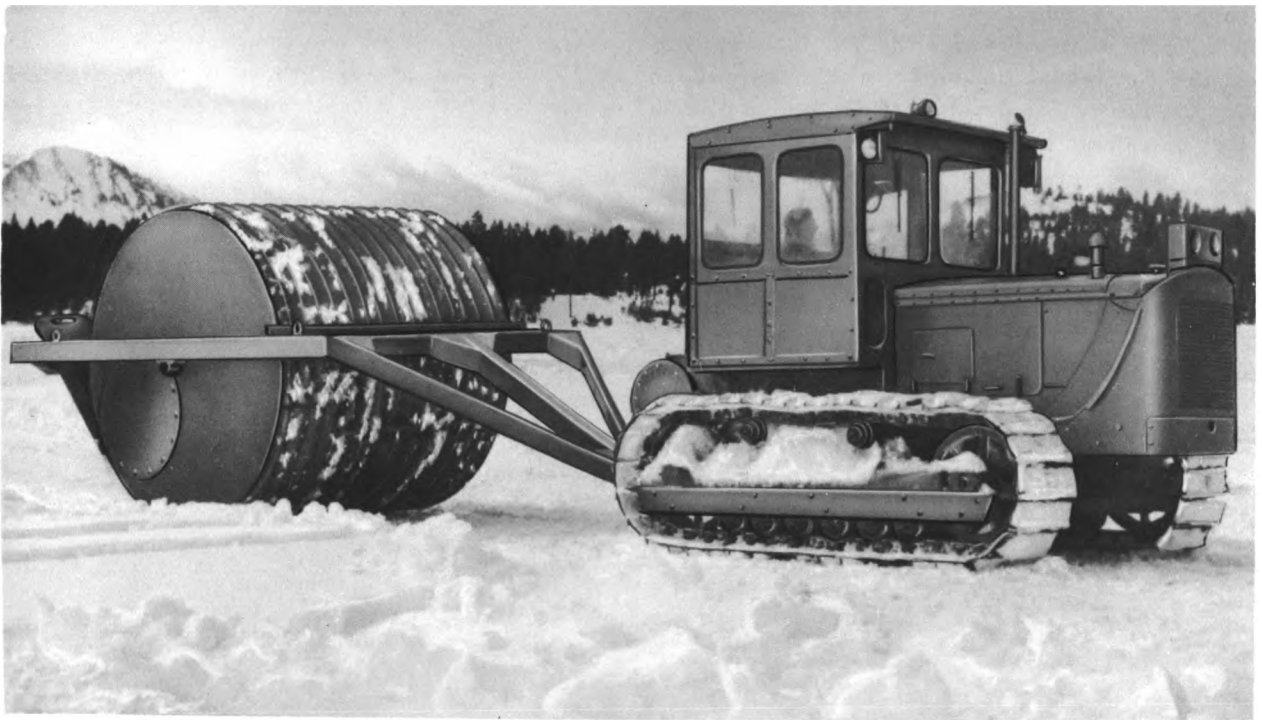
FIGURE 4C2-6 Roller Compacting Snow
