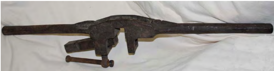
Figure 5.3. Turnbuckle Wrench at Yukon Transportation Museum (Courtesy of Yukon Transportation Museum, Wrench, Tools & Equipment for Materials-Metal Working T&E #2009.31.1)
