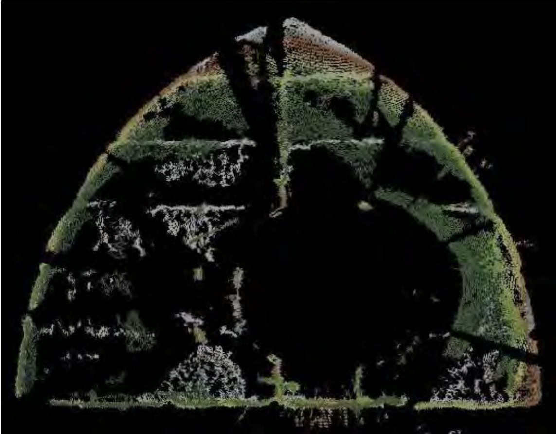
FIGURE 4.10. Interior scan of the A.J. Goddard's bow showing deck beams (Courtesy of BlueView Technologies and OceanGate Inc.).
