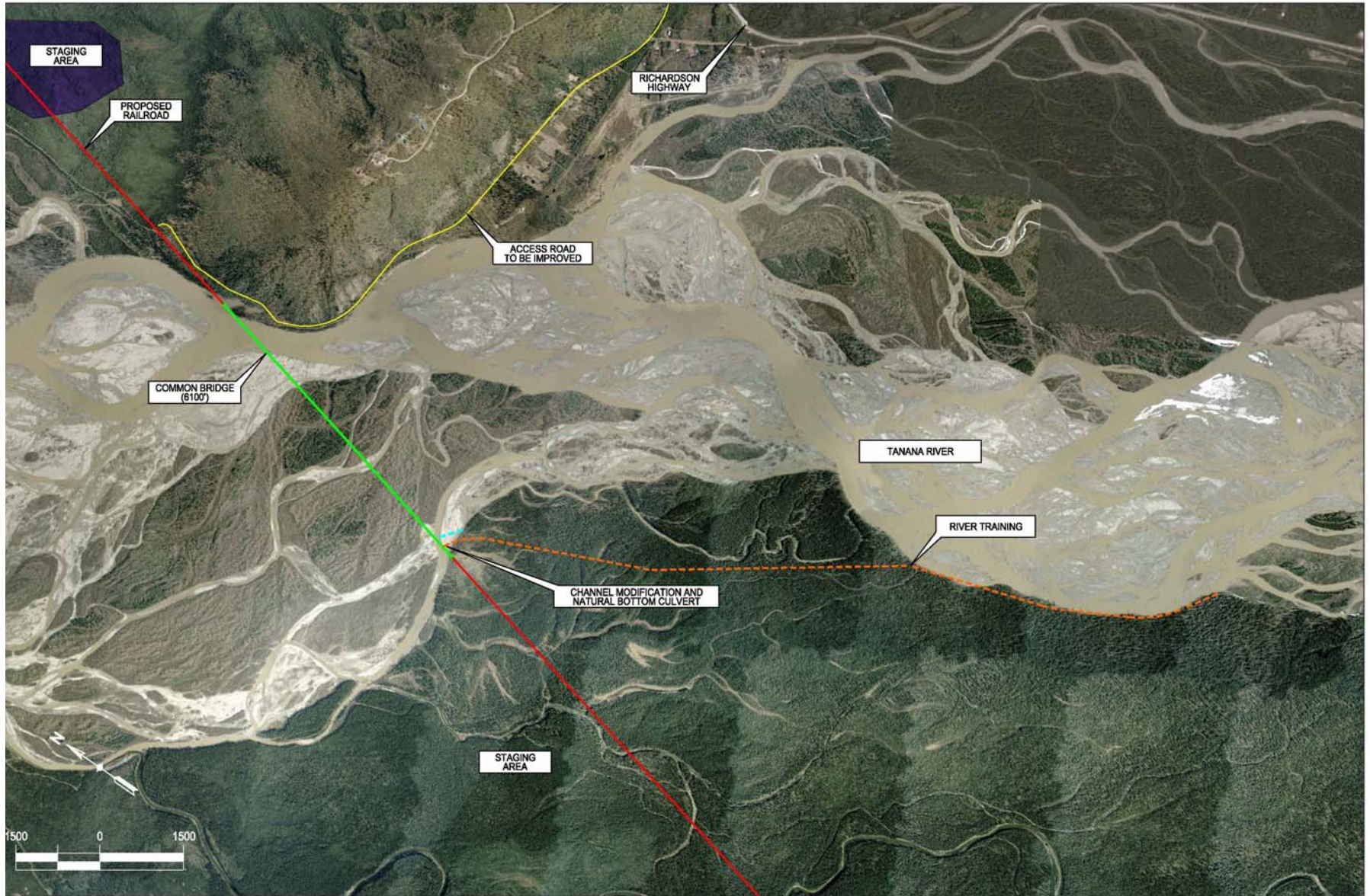
Figure D-4 – Single Bridge Crossing Concept for the Entire Tanana River for Salcha Alternative Segment 2
