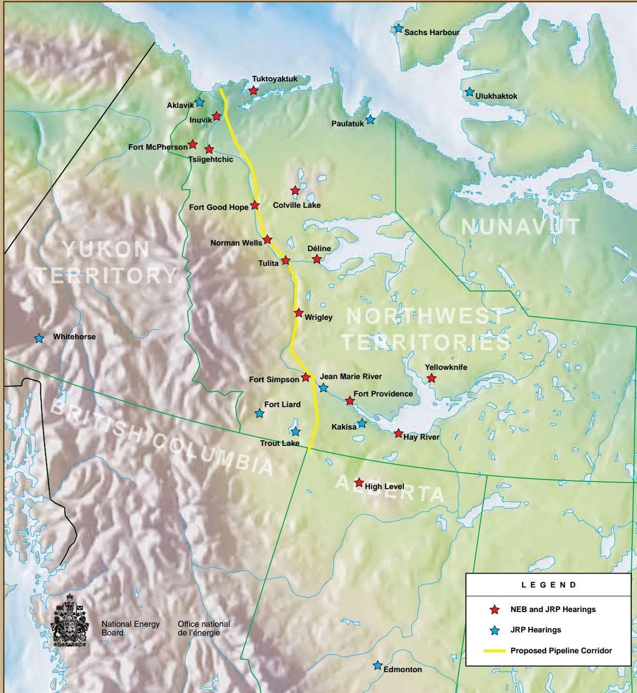
*Proposed to be operational by the end of 2011, the 194-kilometre natural gas pipeline would transport an average 34 million cubic metres (1.2 billion cubic feet) of natural gas per day.*
