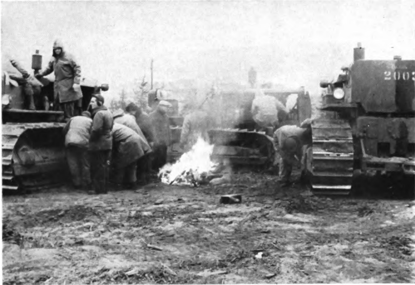
The intense cold caused condensation in fuel lines and stopped the tractors dead.
