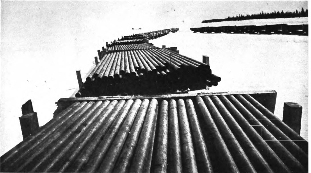
Ingraham Bros. world record load—420 tons over natural ice by one caterpillar D.8 tractor making its own road.
