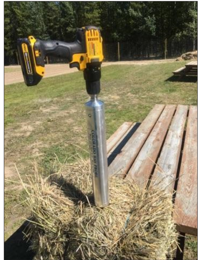
Hay core sampler. This tool takes multiple small samples across different bales which provides a more representative sample from your hay shed.
