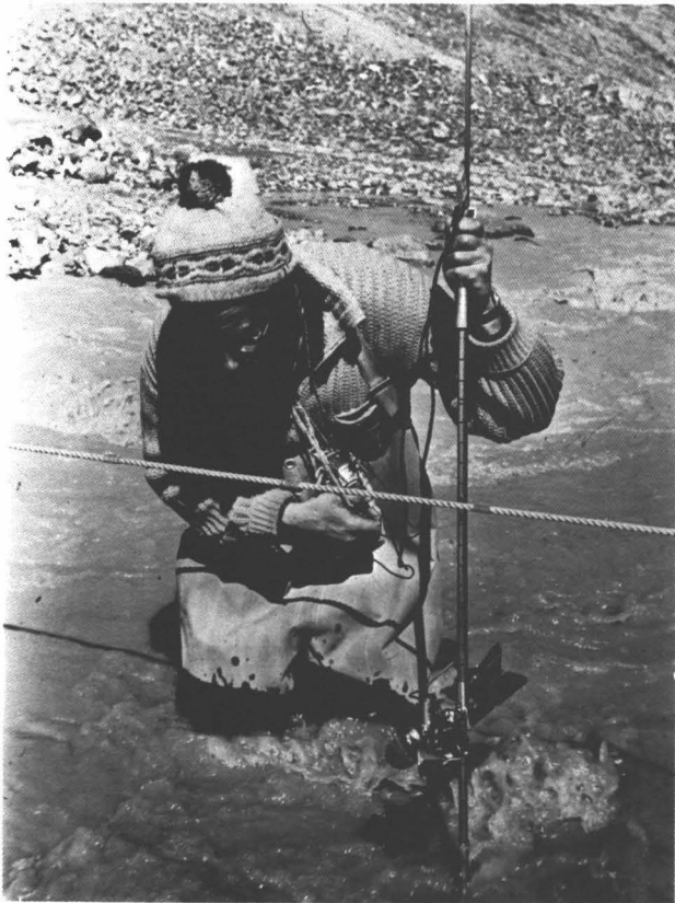
Fig. 5. Current measurement at the site of Rusty I water-level recorder.
