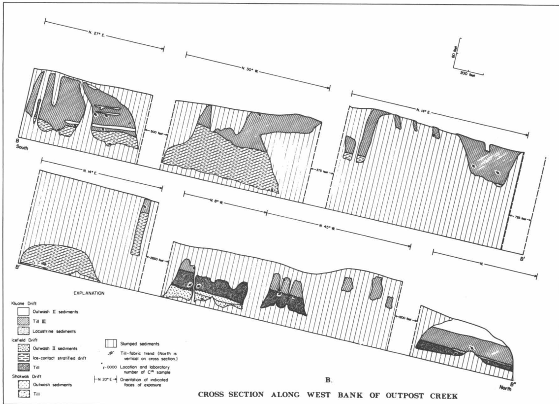
Fig. 5. Cross sections along Silver Creek (A) and Outpost Creek (B), Shakwak Valley. Locations and orientations are designated in Fig. 4. The bottom lines of the cross sections represent the creek beds. Surficial loess units and volcanic ash are not shown.
