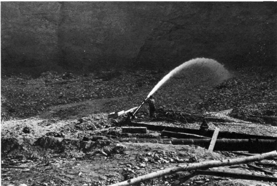
FIGURE 10. Hydraulic mining of White Channel gravels on Cripple Hill.
