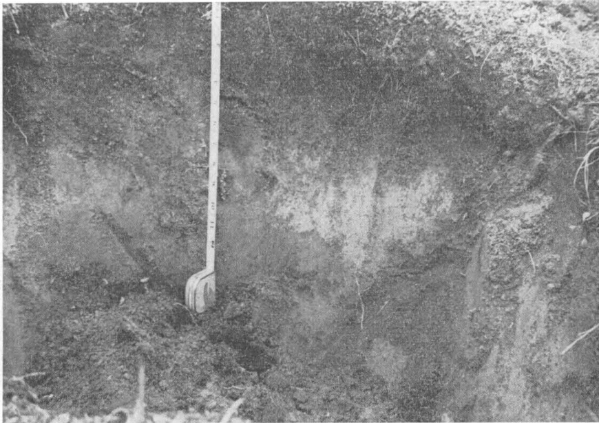
FIGURE 12.—Mendenhall loam has a very dark surface horizon underlain by gray clay. It is a Meadow soil.
