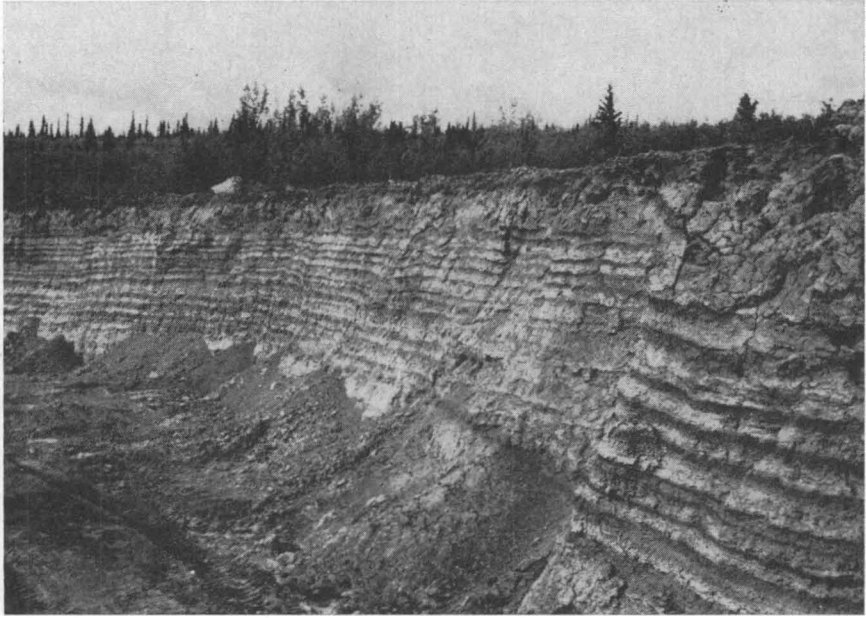
FIGURE 9.—A cross section of the lacustrine silty clay of Glacial Lake Champagne.
