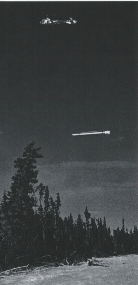
Helicopter-borne magnetic-electromagnetic survey used to detect anomalies.
