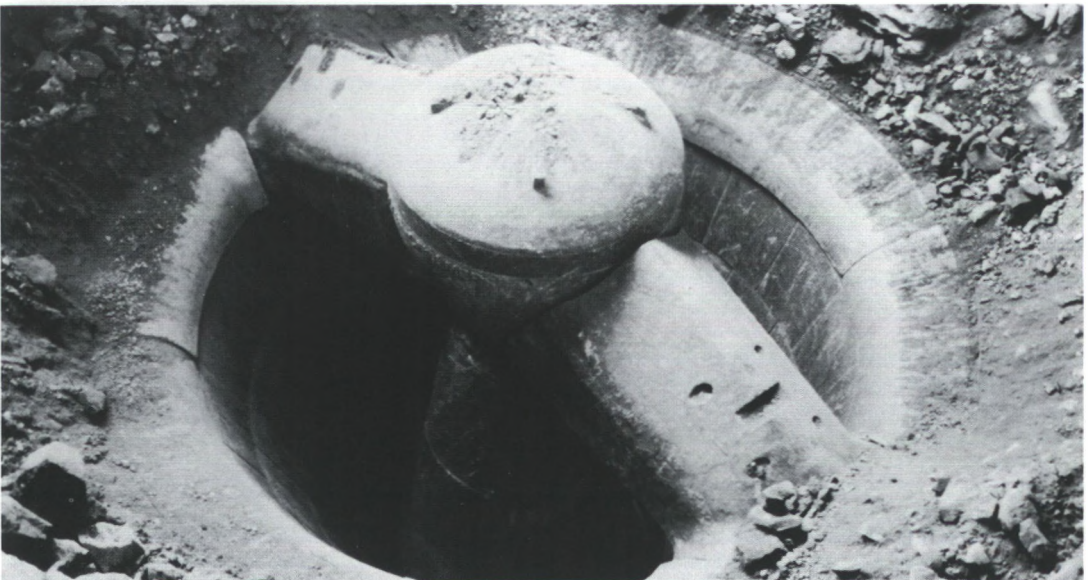
Through the maw of this primary crusher will go 60 million tons of ore.
