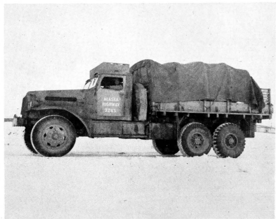
ANOTHER TRUCK built for the desert, but which pounded the icy Arctic trail was the 10-ton White truck, a 6x4 diesel cargo. It taxed skill of driver.
